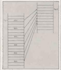
Figure 6. Move one byte in three.
