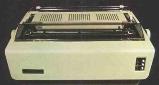
The STARWRITER daisy wheel printer gives top quality printout for any computer with a Parallel or Centronics interface.
