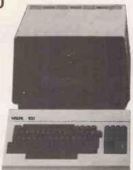
The VISUAL 100 is a new microprocessor based video display terminal that offers total compatibility with the DEC VT100\* from both a software and operator point of view.
