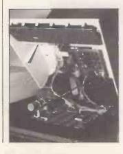
AN RS232 port for the Pet has been developed by Impetus Computer Systems of north London. InPet enables the Pet microcomputer to use a wide range of printers which have the RS232 communications mode. The fully bi-directional InPet allows the Pet to be slowed to wait for the speed of the printer if need be.
