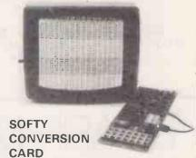
Enables SOFTY to program the single rail EPROMs, 2508/2758/ 2516/2532. Selection of device type and 1K block are by pcb slide switches. Programming socket is zero insertion force. Easy connection to SOFTY with the DEP Jumper supplied. Built and tested: £40+VAT, postage paid.
